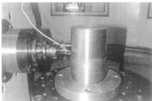
(b) Displacement meter
